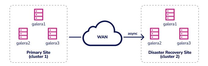
One of the Galera nodes in the DR site would be a slave that replicates from one of the Galera nodes (master) in the primary site. You ship updates on the active cluster asynchronously to the backup site. You could choose to have a dedicated slave instance as the replication relay instead of using one of the Galera nodes as a slave.
