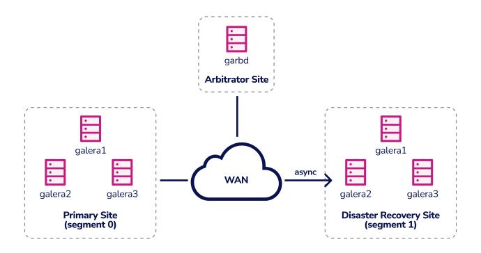
You can also set up an "Active Passive Master-Master Node", where two Galera nodes are located in the primary site, and a third node is located in a disaster recovery site. If the primary site goes down, the cluster will fail as it is out of quorum.
